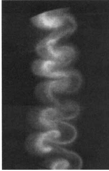
FIGURE 7. PLIF image taken with the laser sheet thickness increased from 0.2 to 2.7 cm in order to demonstrate the two-dimensionality of the flow.
